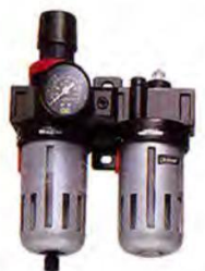
UAC2040B ½" In-line Air Filter / Lubricator / Regulator Auto Drain 5500l/min 10BAR
