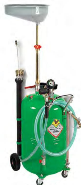
RM44084 Air Operated Waste Oil Evacuator / Drainer Tank - 80L Bowl - 16L Depressurising Pressure - 700 kpa Discharging Pressure - 50 kpa Drain Hose - 2m Suction Time - 2 l/m
