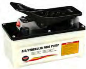
WDA1 Air Hydraulic Foot Pump 10,000 Psi Pressure 1600 ml Oil Capacity 11 in 3 /min Flow ¼" Inlet ⅜" Outlet
