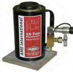
AME13120 55 Ton Hydraulic Jack Ram Min Height 310mm Stroke 150mm - Lightweight Aluminium for Easy Handling - Includes "Shut Off Valve" which Allows Pump to be Removed while Ram is Extended
