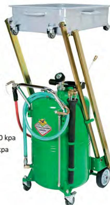
RM44084 Air Operated Waste Oil Evacuator / Drainer Tank - 80L Bowl - 16L Depressurising Pressure - 700 kpa Discharging Pressure - 50 kpa Drain Hose - 2m Suction Time - 2 l/m
