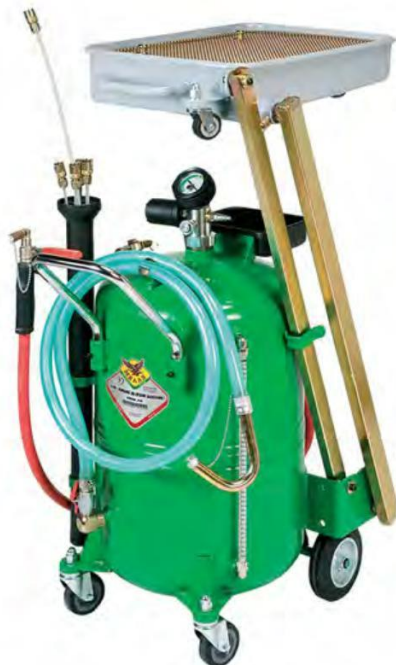
RM46065 Air Operated Waste Oil Evacuator / Drainer Cantilever Type Tank - 65L Bowl - 14L Depressurising Pressure - 700 kpa Discharging Pressure - 50 kpa Drain Hose - 2m Suction Cap - 40L Suction Time - 2 l/m
