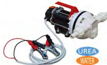
PS204000 12v Urea Pump 36 ℓ/m ¾" In/Out 30 min Duty Cycle
