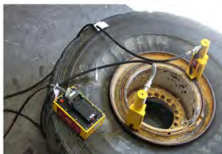
AME12105 Dual Bead Breaker Kit Breaks the Bead on 5 piece Wheel Assemblies at Two Points of Contact. Comes with 3 Hydraulic Hoses & Tee Fitting To Ensure Equal Oil Pressure To Both Units.
